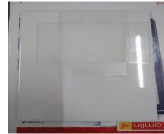
Fig. 7. Deposited polymer after the curing procedure (Ceramic) – 4cmX4cm
