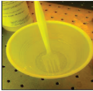
Fig. 3. Mixing of PDMS polymer (Part A and Part B)
